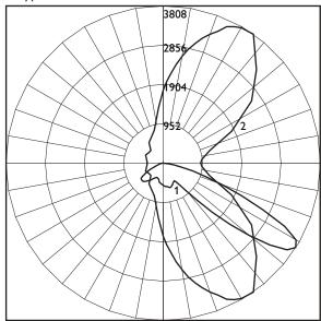
Geoscapes Architectural Wallpack Led - Type Iii (H3) With Individual Led Lens Optics And Clear Flat Glass Lens 54 White Leds. Lumen Output = 4199 Lms.
