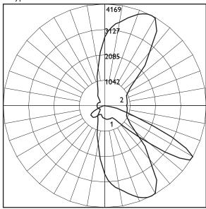
Geoscapes Architectural Wallpack Led - Type Ii (H2) With Individual Led Lens Optics And Clear Flat Glass Lens 54 White Leds. Lumen Output = 4170 Lms.
